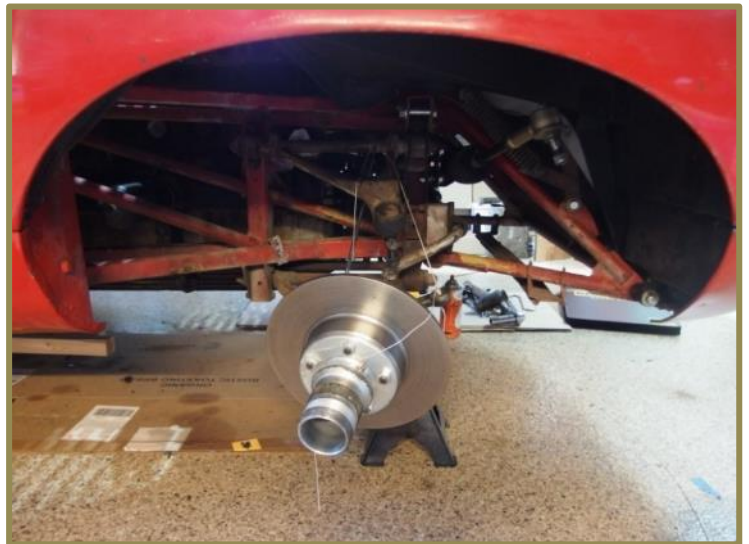
Torsion bars unloaded and suspension hanging loose
