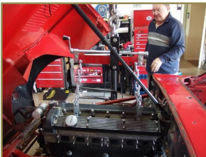
Lift the engine – remove the mounting brackets and lower to the ground!
