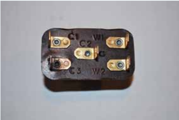
Figure 1. The relay bottom has labels like these. It can save problems later if you note your labels' locations in the comfort of your garage with good lighting. Keep a little diagram in your logbook in your glove box.
