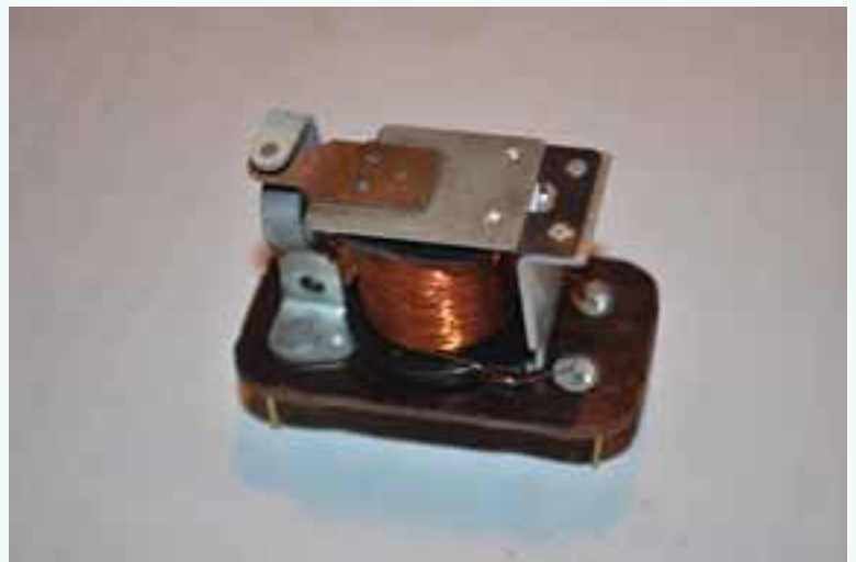
Figure 2. The relay internals are revealed if you unbend some obvious little tabs and remove the cover.
